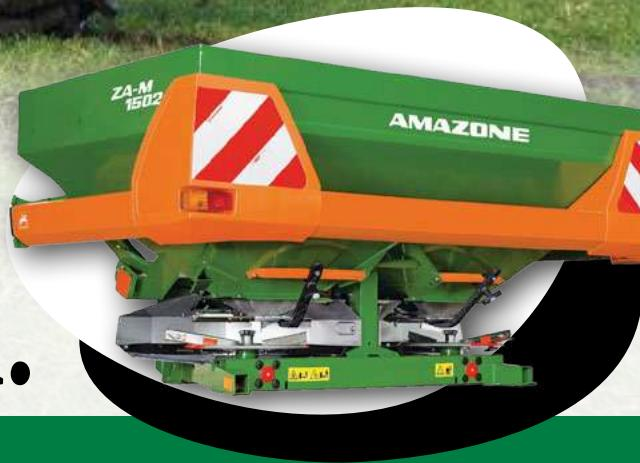
ZA-M 1502 Twin disc Spreader (1 500 ℥) (Excluding Discs) & Spreading disc set OM 10 – 16 m
